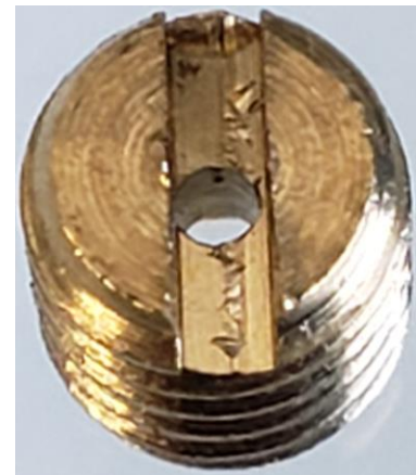
Photo above shows a close up of the screw that has been removed from the snubber and cleaned
