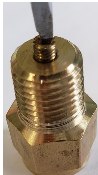
Photo above shows one of the two screws being removed from the snubber
