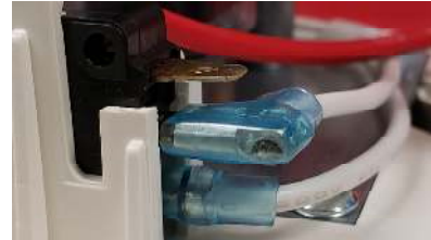
Fig. 5: High level float contacts in N.O. position
