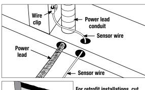
For retrofit installations. cut out drywall and chisel out the bottom plate to route wires to control
